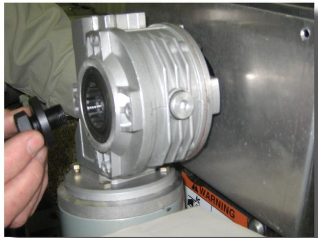
7. Slide the Motor down onto the Spline. Install the Bolt and Washer onto the Motor and Tighten to Approximately 70 Foot Pounds.
