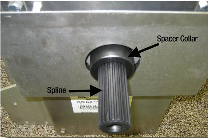
6. Install the Front Cover, Install the Spline, and Install the Spacer Collar.
