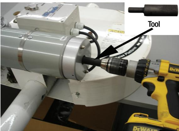
In case of a Power Outage. This Tool may be Inserted into a Drill to Raise or Lower your Lift.
