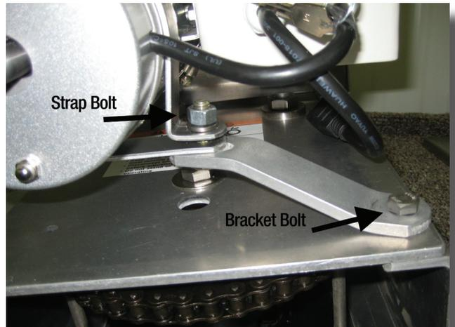
9. Tighten the Strap and Bracket Bolts.
