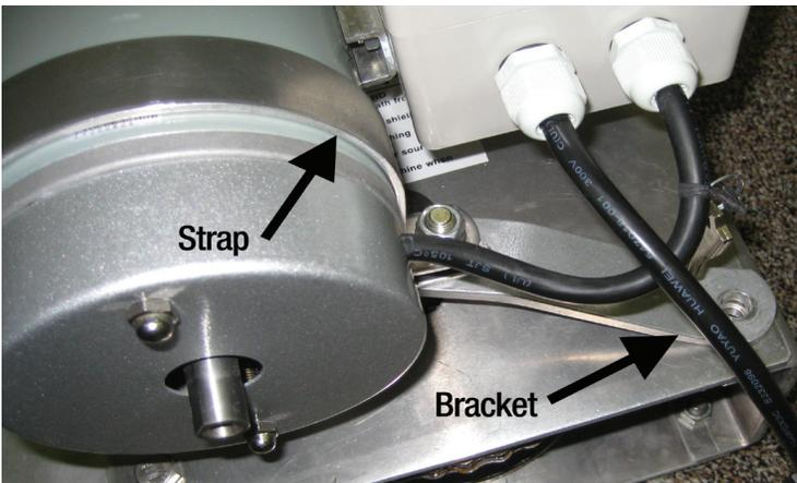
8. Install the Motor Strap around the Motor and Install the Bracket.
