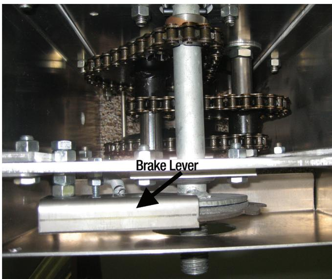
4. Remove the Brake Lever.
