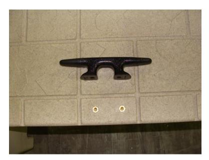
2. Attach the cleat with the  $\frac{1}{4}$  x 2" screws. Be sure to tighten securely.
