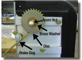
3. Remove the Brake Dog, Brass Washer and the Disc.
