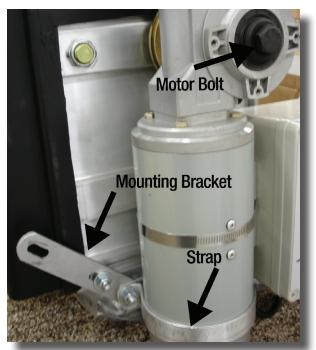
6 .Install the Motor onto the Shaft. Install the Bolt and Washer onto the Motor and Tighten to Approximately 70 Foot Pounds.
