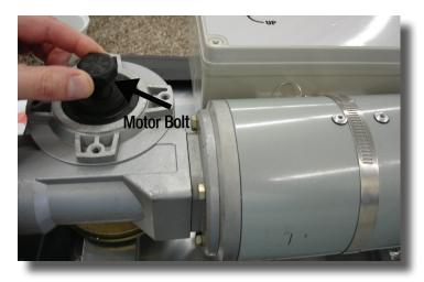
6. Install the Motor onto the Shaft. Install the Bolt and Washer onto the Motor and Tighten to Approximately 70 Foot Pounds.
