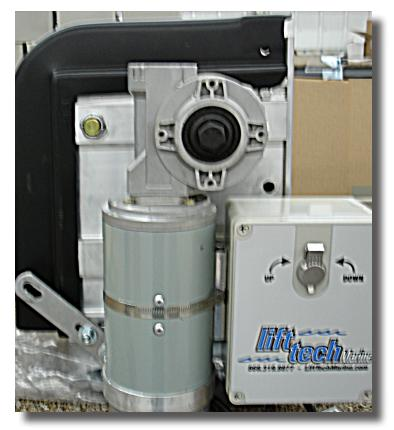
8. Tighten the Strap and Bracket Bolts.
