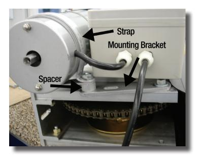
7. Install the motor strap around the motor and connect the strap and bracket with the spacer provided.
