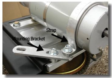
7. Install the motor strap around the motor and connect the strap and bracket with the spacer provided.
