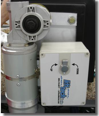
8. Tighten the Strap and Bracket Bolts.
