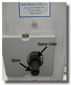
6. Install the Spline, and the Spacer Collar.
