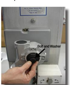
9. Slide the Motor down onto the Spline. Install the Bolt and Washer onto the Motor and Tighten to Approximately 70 Foot Pounds.
