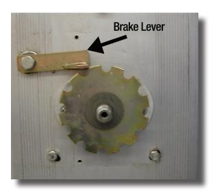
4. Remove the Brake Lever.
