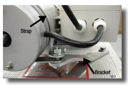
10. Install the Strap around the Motor. Attach the Strap to the Bracket and Tighten all bolts.
