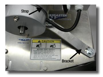
9. Tighten the Strap and Bracket Bolts.
