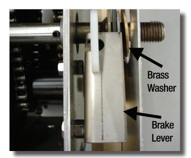
4. Remove the Brake Lever and Brass Washer.
