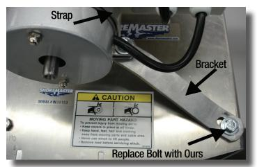
8. Remove the Bottom Right Bolt and Discard the Bolt. Install the Strap around the Motor. Install the Bracket onto the Lift using the Bolt Provided with this Kit.
