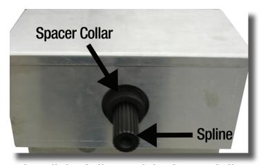
6. Install the Spline, and the Spacer Collar.
