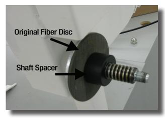
5. Leave the Original Fiber Disc. Install the Shaft Spacer.
