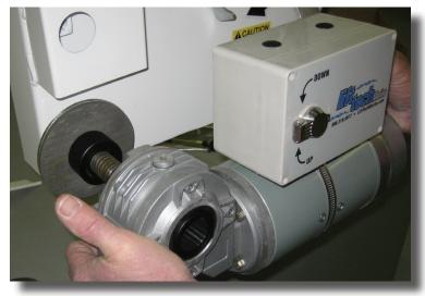
7. Slide the Motor onto the Spline so it sits level.
