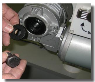
10. Install the Bolt and Washer onto the Motor and Tighten to Approximately 70 Foot Pounds.
