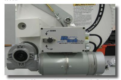
9. Level Motor with Strap and Bracket Installed.
