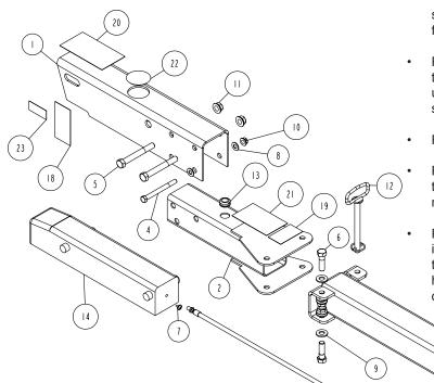
straight tongue. Insert the ½" x 4" hex bolt and secure with a ½" flange lock nut.
