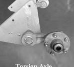
**Torsion Axle** 3750# Torsion axle, Galvanized Axle Body, Arm, and Hubs, Sure Lube Hubs
