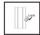
Secure each arm assembly by locking the travel lock. Push down on the travel lock assembly to secure. The awning is now completely closed and ready for travel.
