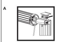
Remove Patio O'Shade if installed. In one hand gently pull on the pull strap while using the pull rod to flip the Safe-T-Lock™ Lever up into the "ROLL UP" position.
