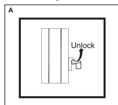
Unlock the travel lock located mid way up each arm assembly. Lift up on the travel lock assembly to unlock.
