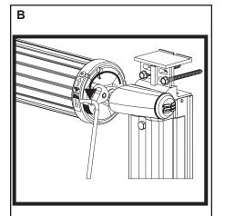
Use the pull rod provided to rotate the Safe-T-Lock™ Lever down to the "ROLL DOWN" position.
