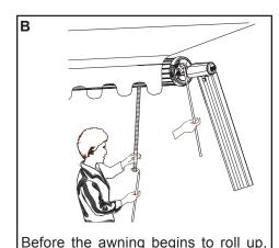
insert end of pull rod into the pull strap
